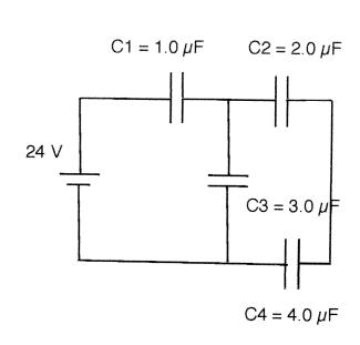
$$\Delta V_{234} = \frac{Q_{234}}{C_{234}} = 4.5 \text{ Volts}$$
