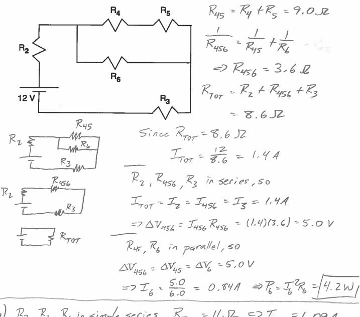
b)  $R_2$ ,  $R_3$ ,  $R_6$  in simple series.  $R_{Tor} = 1/JZ = 5I_{Tor} = 1.09A$   $I_{Tot} = I_2 = I_6 = I_3 = 5I_6 = 1.09A$   $P_6 = I_6^2 R_6 = 7.1W / increases /$
