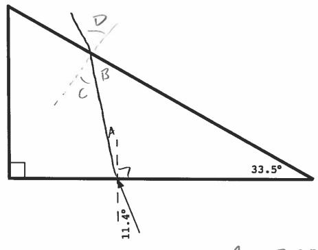
1.0 sin 11.4 = 1.44 sin  $A = A = 7.9^{\circ}$   $A + 90^{\circ} + 33.5^{\circ} + B = 180^{\circ} = B = 48.6^{\circ}$   $B + C = 90^{\circ} = C = 41.4^{\circ}$ 1.44 sin  $C = 1.0 \text{ sin } D = D = 72.2^{\circ}$
