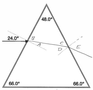
$\frac{B/ue}{1.0 \sin 24^\circ = 1.48 \sin A}$   $=> A = 15.95^\circ$   $A+B=90 => B = 74.05^\circ$   $B+48+C=180 => C = 57.95^\circ$   $C+D=90 => D = 32.05^\circ$   $1.48 \sin 32.05^\circ = 1.0 \sin E$   $E = 51.75^\circ$
