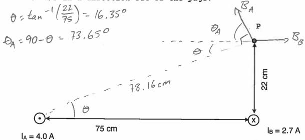
$$\begin{array}{ll} A = 4.0 \, \text{A} \\ \hline a \\ \end{array} & (B_A )^{-} \frac{M_o (4)}{2\pi (.7816)} = 1,024 \, \text{mT} \qquad B_{A_X} = -1,024 \, \cos 73.65^{\circ} \\ & = -0,288 \\ |B_B| = \frac{M_o (2.7)}{2\pi (.22)} = 2.45 \, \text{mT}_{,+\chi} \qquad B_{A_Y} = +1,024 \, \sin 73.65^{\circ} \\ & = 0,982 \end{array}$$
