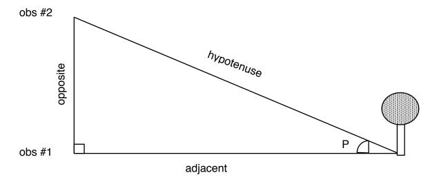
If we physically walk from observation point #1 to observation point #2, then we know that distance. Let's assume it is 25 meters. Using a protractor or other angular measuring device, we can also determine angle P. Let's assume that angle P is 27 degrees.
