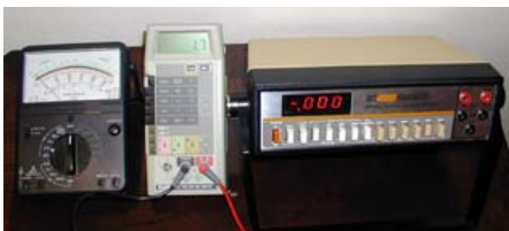
Figure 2.1: Multimeters Typical analog (left) and digital multimeters (center and right).
